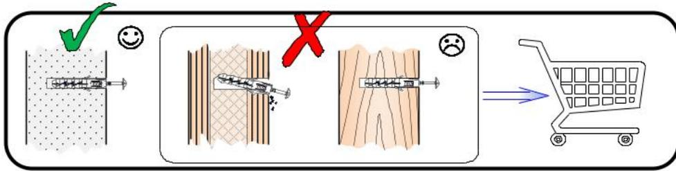
**EN** Before suspending or fixing furniture to the wall (in order to prevent falling over), check the type and strength of the wall. Select wall plugs and screws appropriate for the given type of the wall. In the case of doubts, contact a specialist. The installation must be performed by a competent person. **WARNING!!!** If the rawlplugs with screws are attached to the product, then they are intended only for walls made of solid and homogeneous materials.
